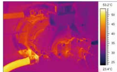
Limited temperature increase of only 25° C inside compressor element
